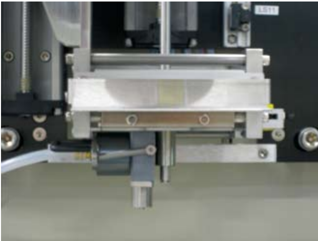
Solder Scavenger with Dynamic Height Sensing Automatic non-contact solder removal
